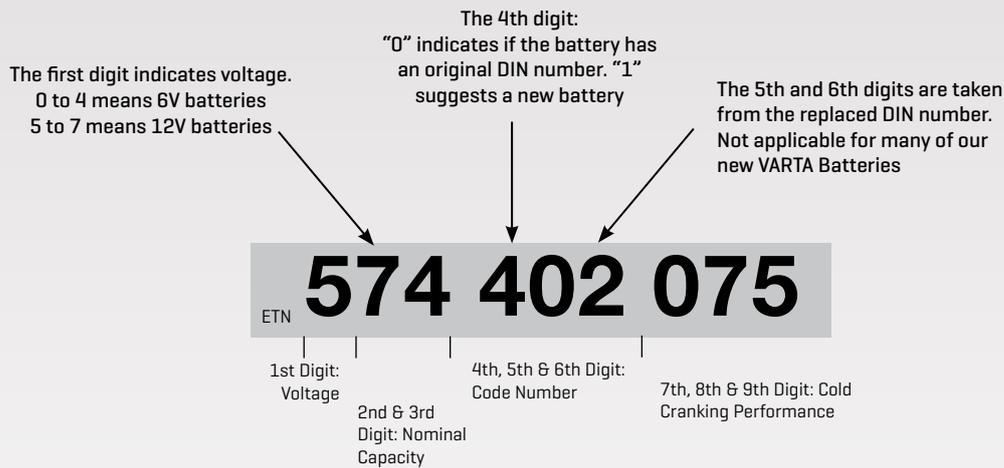
The 2nd and 3rd digits indicate nominal capacity. For batteries with a capacity above 100A/Hrs, the first digit increases by 1.
